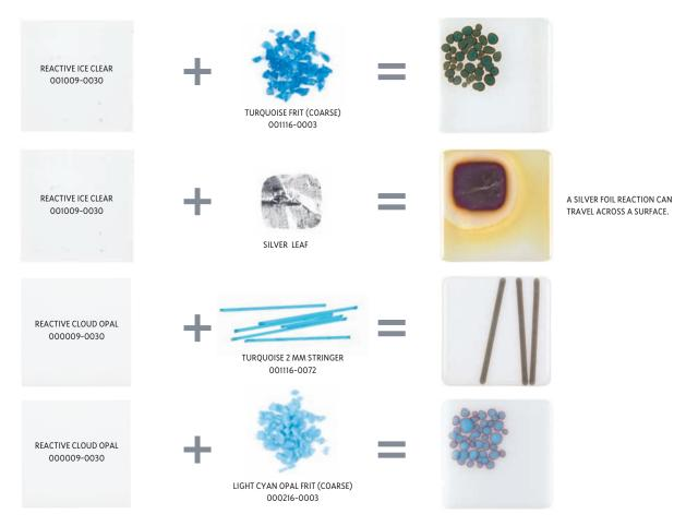
LAYUPS: 6MM STACKS (3MM CLEAR BASE + 3 MM REACTIVE SHEET), -0003 FRIT, 2MM STRINGER, BULLSEYE SILVER FOIL. PROCESS TEMPERATURE: 1480°F (804°C)
